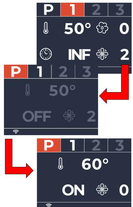
When the oven temperature reaches the selected preheating set point, an acoustic alarm is activated to warn of this event. To interrupt this alarm, simply press any button or open the oven door.
