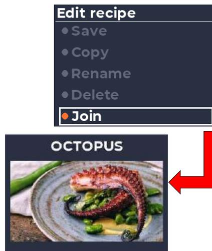
There is the possibility of assigning an image that does not exist in the library already available in the furnace. To do this, the image must be saved on a USB storage device, which must contain in its root directory ONLY a folder named "jpg", and where the desired images must be placed.
